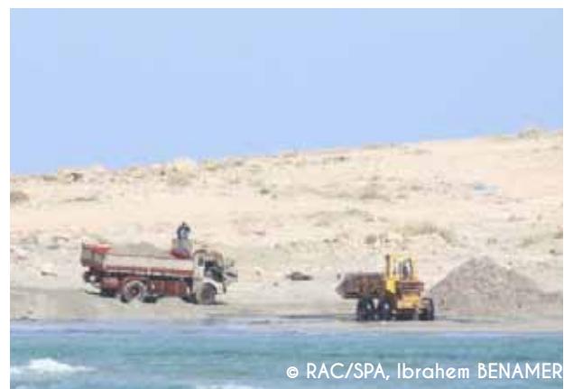
Figure 13. Sand dredging operations with heavy machinery. A truck shown in the picture is loading up sand to be carried to nearby urban areas
