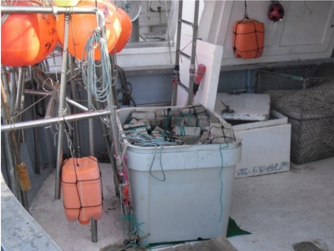
Figure 50. Basket full of stones used as leads by a longliners.
