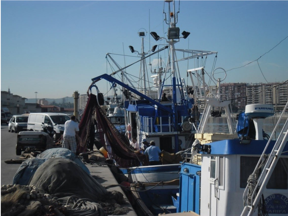
Figure 40. Purse seiners with one simple hauler from port of Algeciras (Spain).
