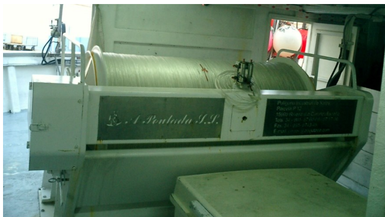
Figure 45. Hydraulic reel, where the mainline is stored.
