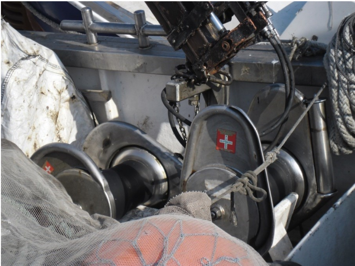
Figure 41. Purse seiners with one complex hauler (port of Carboneras, Spain).
